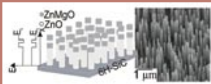
Figure 1: Sketch of ZnO/ZnMgO quantum well structures realised on ZnO nanorods (SEM image of nanorods on the right)
